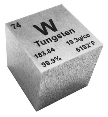
Tungsten is a rare and valuable metal, primarily used in applications requiring high strength and heat resistance, such as in lightbulb filaments, aerospace components, and military applications.
